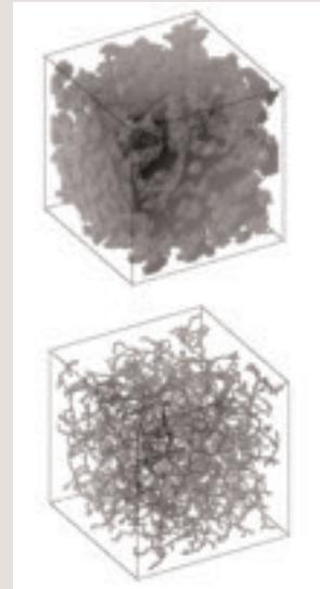
> 3D reconstruction of the topological skeleton (bottom) characterizing a granular porous mineral (top).
