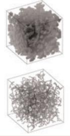
> 3D reconstruction of the topological skeleton (bottom) characterizing a granular porous mineral (top).
